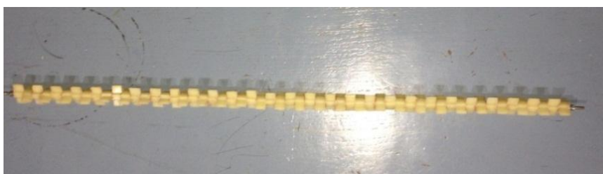
Fig.1. a) Photograph of experimental setup b) Nylon flow divider insert
